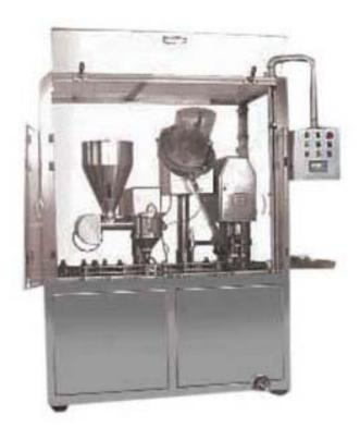
The Automatic Dry Powder Filling with ROPP/Screw/CRC Capping Machine is a combination of Auger type Powder Filling with Capping machine. It is available in 2 models i.e.
